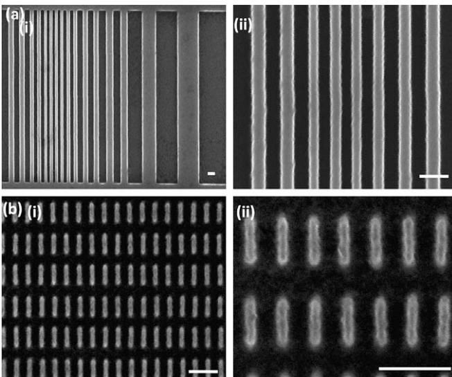
Fig. 2. SEM measurements of silicon masters: (a) PMMA-master with widths varying from 1  $\mu\text{m}$  to sub-100 nm, (i) survey, (ii) zoom on smallest structures, (b) HSQ-master with sub-50 nm structures (i) survey, (ii) zoom; scale bars correspond to 200 nm.
