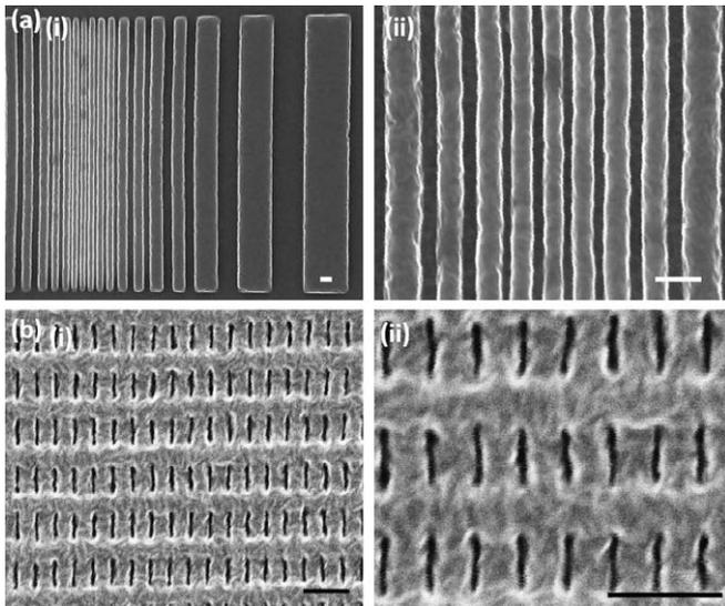
**Fig. 3.** SEM measurements of Surlyn molds: (a) Protrusion mold with widths varying from 1  $\mu\text{m}$  to sub-100 nm, (i) survey, (ii) zoom on smallest structures, (b) cavity mold with sub-50 nm structures (i) survey, (ii) zoom; scale bars correspond to 200 nm.
