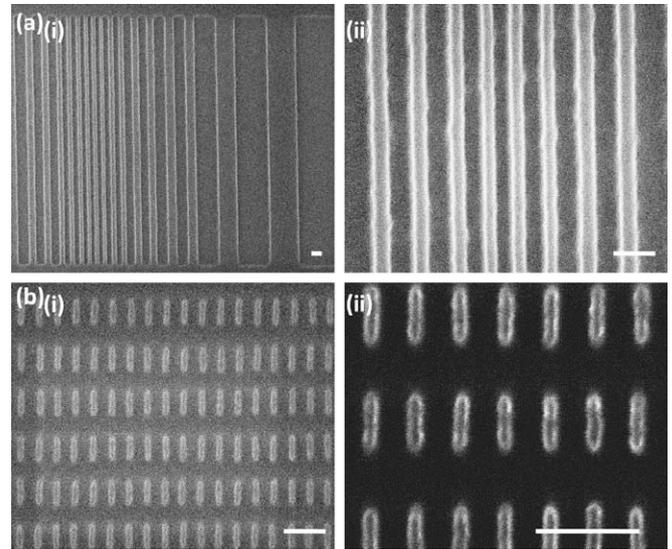
**Fig. 4.** SEM measurements of imprints with Surlyn molds in UV resist: (a) Cavity imprint with widths varying from 1  $\mu\text{m}$  to sub-100 nm, (i) survey, (ii) zoom on smallest structures, (b) protrusion imprint with sub-50 nm structures, (i) survey, (ii) zoom; scale bars correspond to 200 nm.
