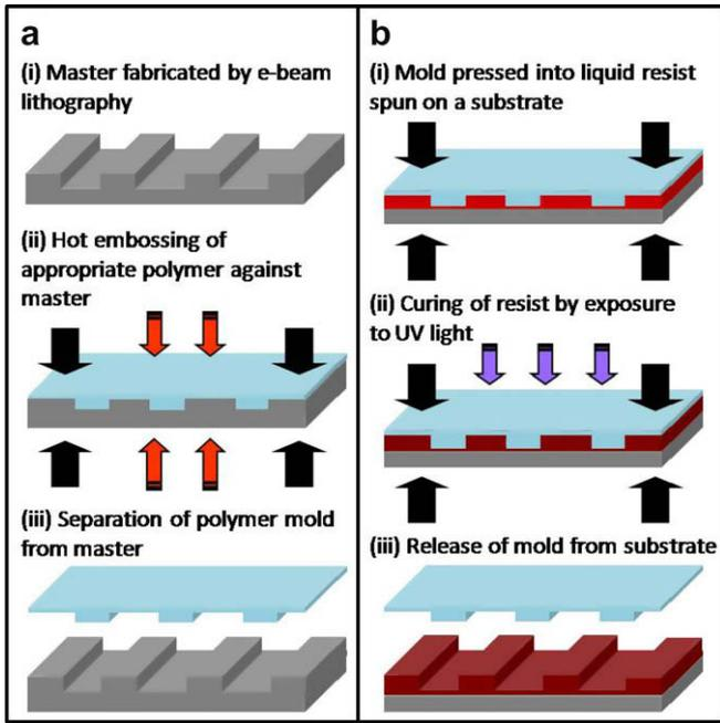
Fig. 1. Schematic process of (a) polymer mold fabrication from a master and (b) UV nanoimprint with the polymer mold.
